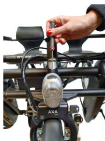
Headlight hook up and closing
