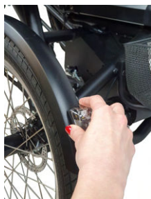
Get bulb holder straight to rear loose
