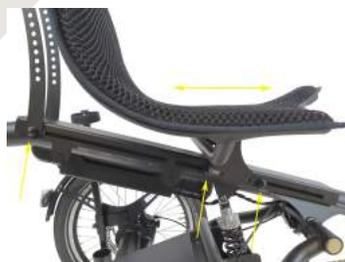
The height of the seat changes automatically when the seat depth is adjusted, because the mounting tube runs diagonally upwards. When the seat depth is adjusted correctly, the seat height will automatically be right. With the seat in the right position, you will effortlessly pedal away the kilometres.
