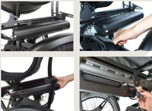
1. Attach the adapter to the charging plug.
