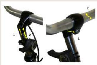
Adjusting handlebar height and angle
