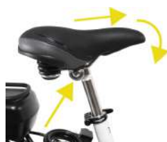
Adjusting saddle depth and angle
