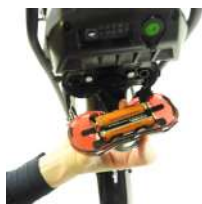
Take off the rear light and replace batteries
