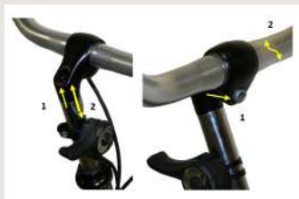
Adjust handlebar height Adjust steering angle
