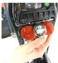
Push the black locking device downwards
