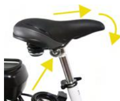
Adjusting saddle depth and angle
