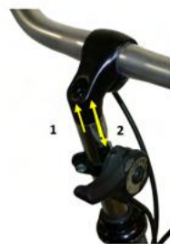
Adjust handlebar height
