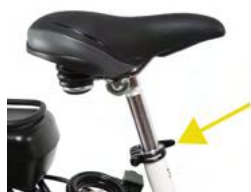
Seat height via quick-release lever
