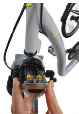
Unscrew bulb holder straight back
