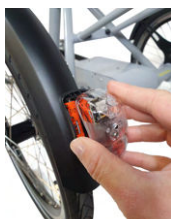
Unscrew bulb holder straight back
