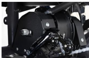
Motor in achter frame
