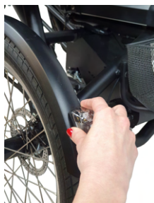
Get bulb holder straight to rear loose
