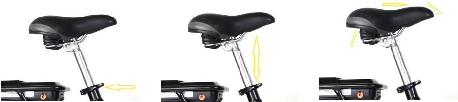
Saddle height with quick tensioner
