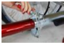
Lift the frame out of the lock
