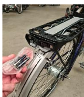
Changes batteries. Mind the + and – of the batteries
