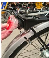
Hook in the back light and push to lock.
